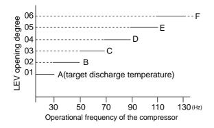
In COOL operation, the two indoor coil thermistors (one main and one sub) sense temperature ununiformity (super heat) at the heat exchanger, and when temperature difference have developed, the indoor coil thermistors adjust LEV opening degree to get approximate 10 degrees lower temperature than the target temperature in the table above, thus diminishing super heat.
